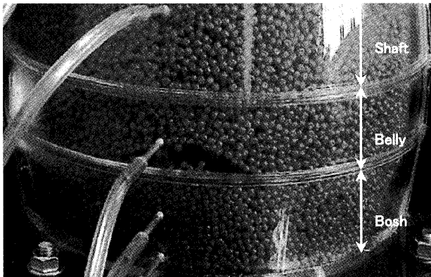
Fig. 8. Collapsing bridge at Belly in the case of Fig. 7.
