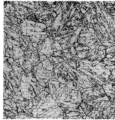
Fig. 1. Optical micrograph of specimen, ASME Gr.92 steel.
