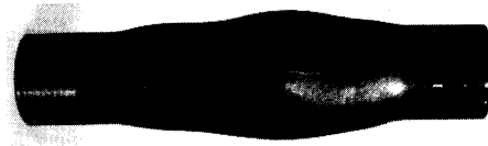
Fig. 8. Bulge formed shape of a cold-drawn and normalized specimen (No. 3).
