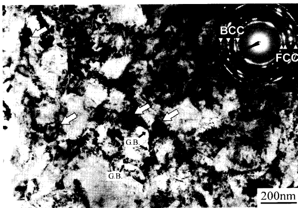
Fig. 3. TEM micrograph and the SADP of an inner region of the powder milled for 720 ks. Arrows indicate spherical fine grains.
