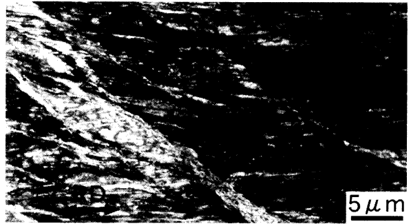
Fig. 6. TEM micrograph (bright-field) of SUS310S specimen cold-rolled by 70% in thickness reduction.
