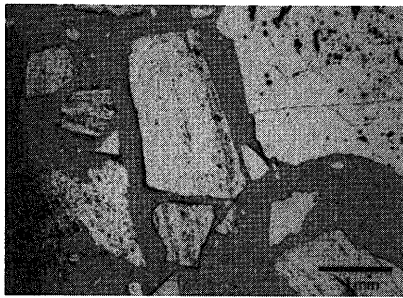
Photo a-1 (X25) Coarse coal sample -- many cracks caused by the rapid heating
