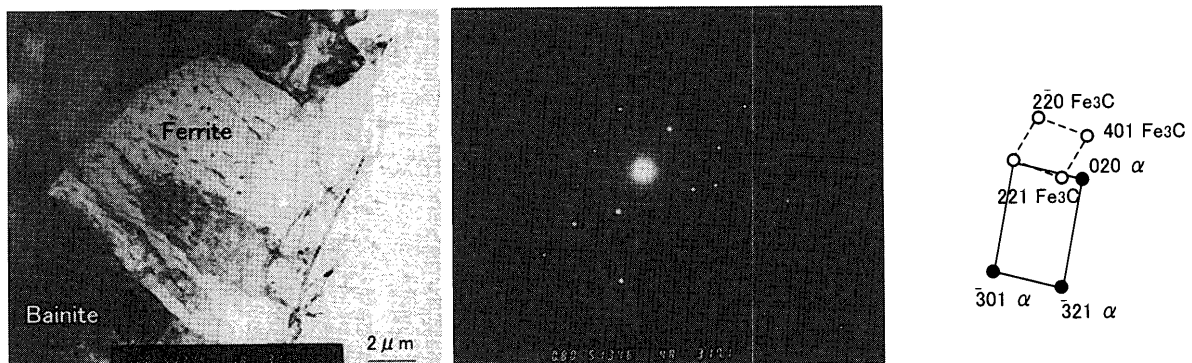
Fig. 12. TEM bright field image (a) and diffraction pattern (b) confirming the existence of cementite in DIDT ferrite.
