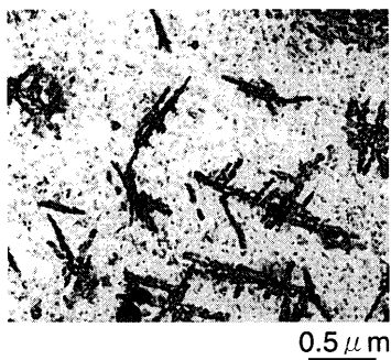
Fig. 12. Extraction replica image of nitrided 11% Cr steel (11%Cr-0.4%Mo-2%W-1%Cu-Nb-V steel). 773K for 54 ks, N 2 :H 2 =1:1, 900-1100 Pa.
