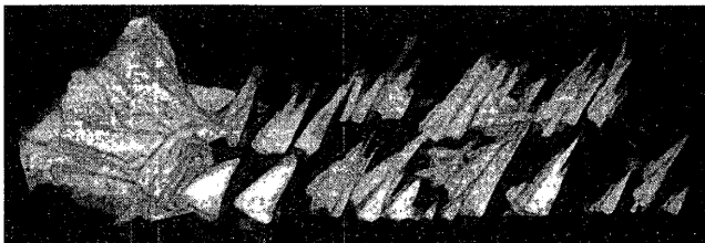
Fig. 3. 3D-reconstructed image of ferrite precipitates at austenite grain boundaries in an Fe-0.12wt%C-3.28wt%Ni alloy austenitized at 1100°C for 30 s and isothermally reacted at 650°C for 2~3 s. 17) The length of the bottom side is about 100 μm.
