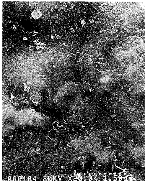
Fig. 12. SEM microphotographs of discolored Ti roof exposed for 10 years.
