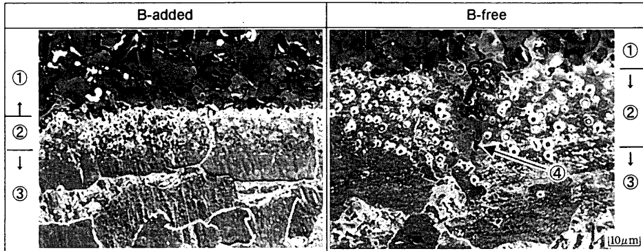
Fig. 3. SEM at cross section of steels forged at 1200°C.
