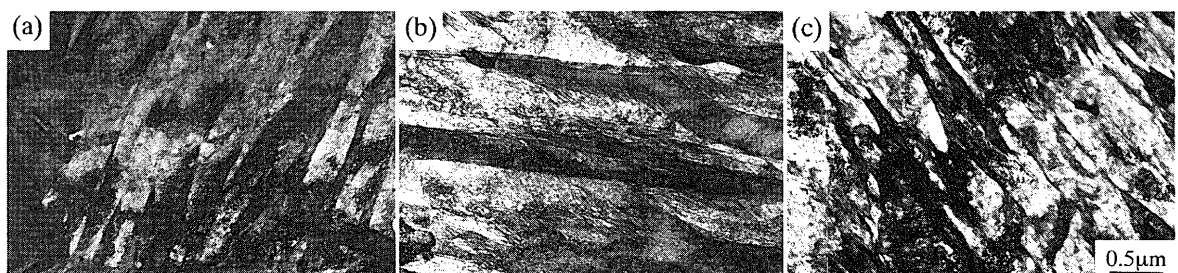
Fig. 2. Transmission electron micrographs showing martensite lath structure in (a) 9Ni, (b) 9Ni-1Cu and (c) 9Ni-3Cu steels.
