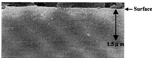
Fig. 6. SEM morphology of cross section of the cold rolled sheet (Steel A).
