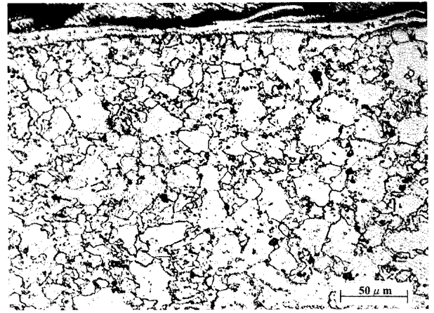
Fig. 17. Feature of Type IV damage near the top surface. (Sectioned after failure.)
