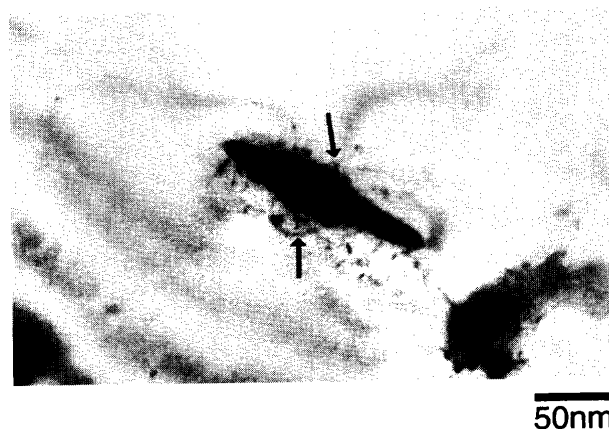
Fig. 10. TEM micrograph showing the interface dislocations around the fine Laves phase precipitated in S8C46W steel in the as-tempered state. Morphological change from the plate-like to granular shape is seen in the part of the Laves phase surrounding by the dislocations as indicated by arrows.
