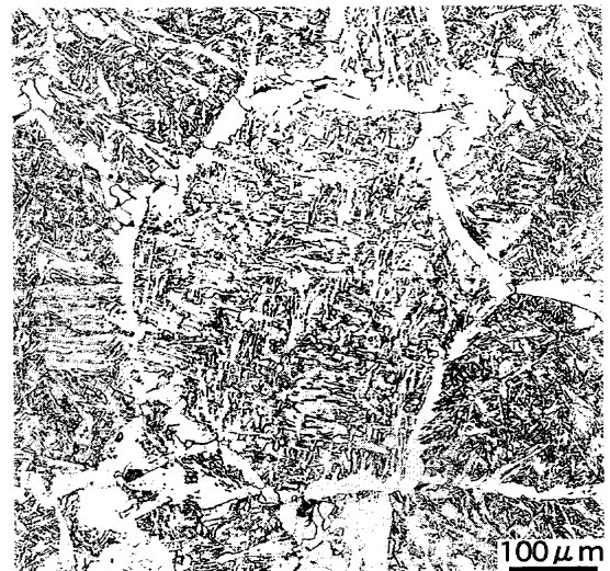
Fig. 4. Optical microstructure of sample continuously cooled from 1673K.
