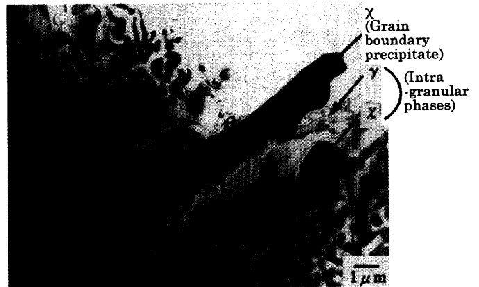
Fig. 5. Phase identification result of 12MLN by TEM.
