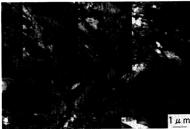
Fig. 1. Bright field TEM image of a modified 9Cr-1Mo steel in the as received condition.
