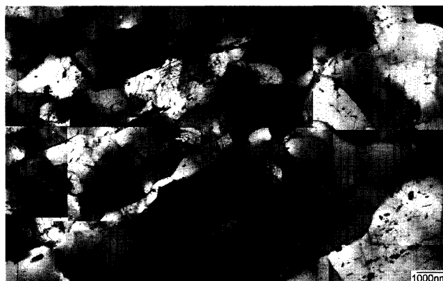
Fig. 9. Bright field TEM image of BT specimen creep ruptured after 26517.1 h at 848K-59 MPa.
