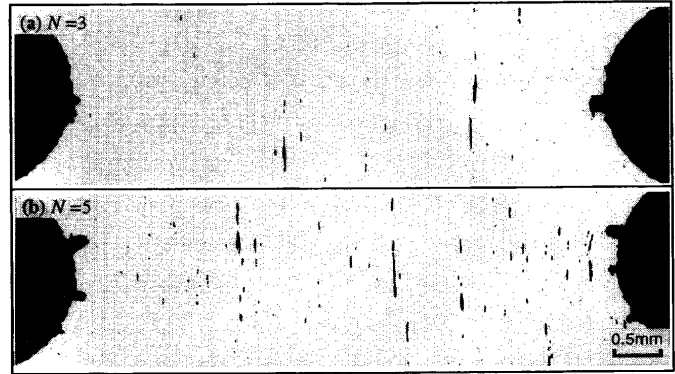
Fig. 14. Void growth during cyclic loading in Steel B ( \rho=1.0\text{mm} , \varepsilon_a=1.0\% ).
