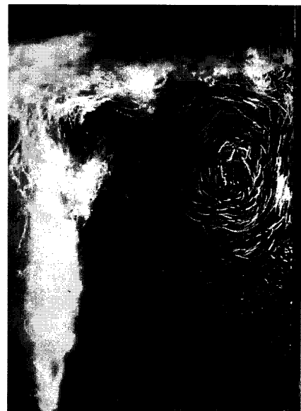
Fig. 2. Visualized flow pattern. (q G = 167 × 10 -6 m 3 s -1 )
