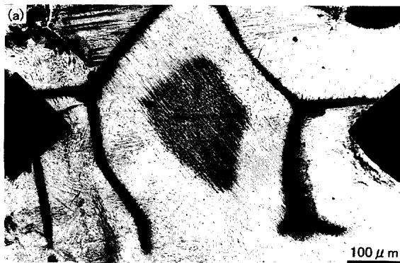
Fig. 5. Microstructure of fine columnar \gamma grain region.
