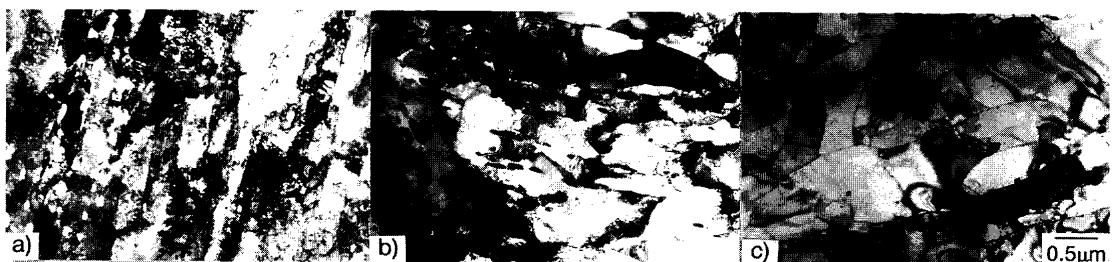
Fig. 5. TEM thin-foil micrographs showing martensite structure at each tempering temperature: (a) 730°C-10 h, (b) 760°C-20 h, (c) 780°C-20 h.
