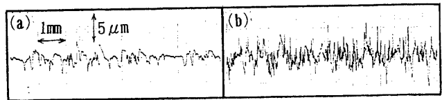
(a) GI with resin coating 1.4g/m 2 (b) GA with resin coating 1.4g/m 2
