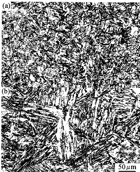
Fig. 8. Optical micrographs of specimen No. 11 austenitized at (a) 1273K and (b) 1473K.
