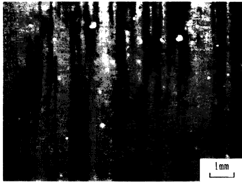
Fig. 2-(c). Roll surface of banding area (The scale is partially peeled off).
