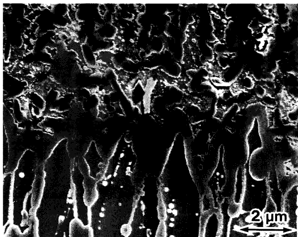
Fig. 2. Structure at near the top of remained \zeta ・Fe-Zn phase. (Coating obtained by immersing HDG-3M specimen for 1 s in Zn-5mass%Al bath at 450°C.)
