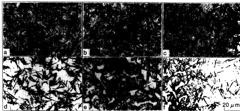
(a) 1.00%Cr(D1), CP=0.75% (b) 1.53%Cr, CP=0.75% (c) 0.99%Cr-0.80%Mo, CP=0.75% (d) 1.00%Cr(D1), CP=1.16% (e) 1.53%Cr, CP=1.16% (f) 0.99%Cr-0.80%Mo, CP=1.16%
