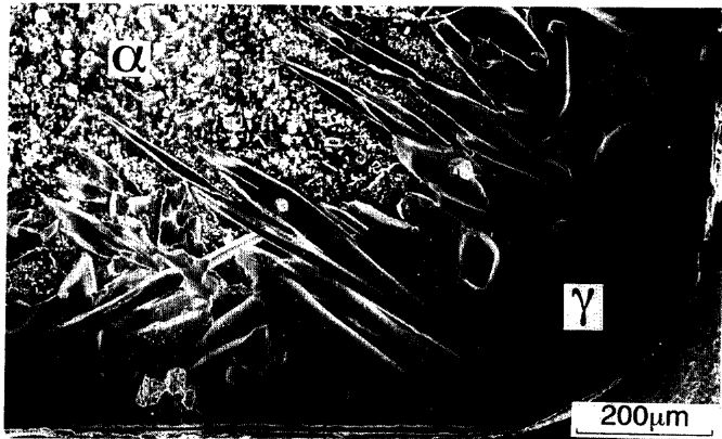
Fig. 3. SEM image showing the microstructure of Fe-27mass%Cr alloy with nitrogen absorption treatment. Treated at 1473K for 16.2 ks in 1 atm \text{N}_2 gas atmosphere.
