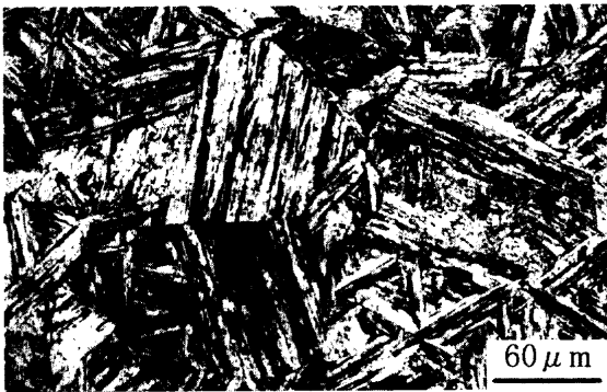
Fig. 4. Microstructure of the specimen quenched and kept at 313K after solution treatment and aged at 753K for 14.4ks.
