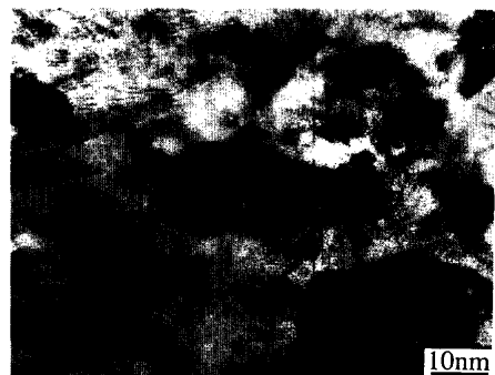
Fig. 8. TEM micrograph of a 720ks MM powder. The powder to ball ratio was 1:12.
