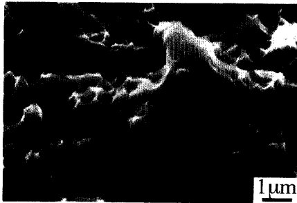
Fig. 13. A slant view of the fracture surface of a HIP compact tensile tested at R.T.
