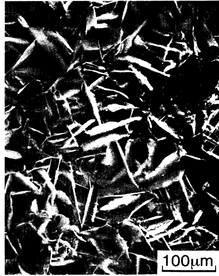
Fig. 9. Scanning electron micrograph of 13mass%Mn-0.9mass%C steel isothermally transformed at 793K for 5.4ks. The specimen was deeply etched by 3% nital to make the morphology of platelet carbide clear.
