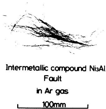
Fig. 6. An example of fault Ni 3 Al filament produced in Ar gas.
