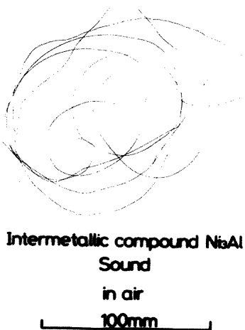
Fig. 7. An example of sound Ni 3 Al filament produced in open air.
