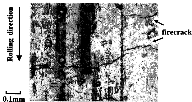
Fig. 8. Optical micrograph of worn surface of high Cr cast iron. A lot of firecracks exist, which is perpendicular to rolling direction.
