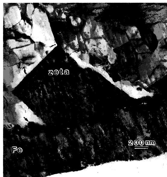
Fig. 10. TEM bright field image of cross section of \zeta -ZnFe alloy formed in 0.086 mass% phosphorus added steel sheet. Al content in zinc bath was 0.12 mass% and steel was immersed at 733 K for 3 sec. Arrow: Al-Fe alloy, zeta: \zeta -ZnFe alloy, Fe: steel substrate.
