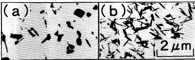
Fig. 1. Transmission electron micrographs of extraction replicas of 2.25Cr-1Mo steels used in an actual boiler. (a) Sample A1 used at 843K for 3.58 \times 10^8 s. (b) Sample B1 used at 866K for 3.58 \times 10^8 s.
