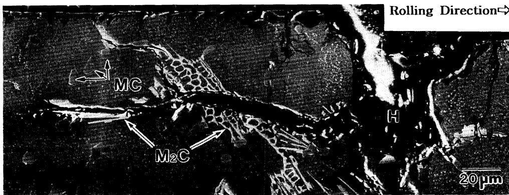
Fig. 3. SEM micrograph of the near-surface region of the sectioned A-roll specimen, showing black oxide layer, coarse carbides, and cracks.
