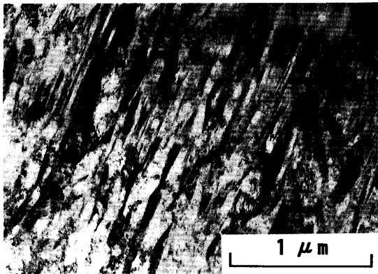
Fig. 4. TEM microstructure of deformation induced martensite aged at 400°C for 3.6ks after 50% cold rolling in A steel.
