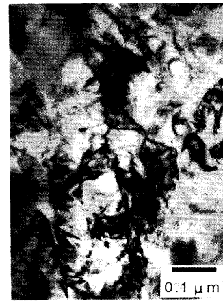
Fig. 4. TEM of a thin foil of the mechanically alloyed (MA) 13%Cr-3%Ti-3%Y _2 O _3 steel powder. (MA for 48h, The thin foil is prepared by an ion milling.)
