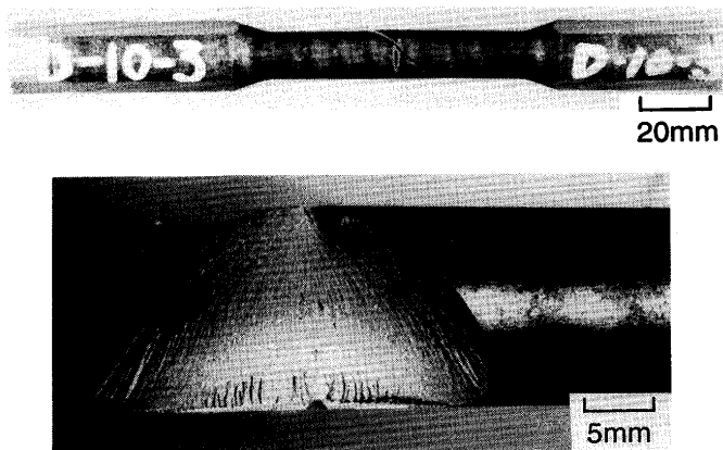
Fig. 2. Macroscopic view of fractured specimen (steel A6).
