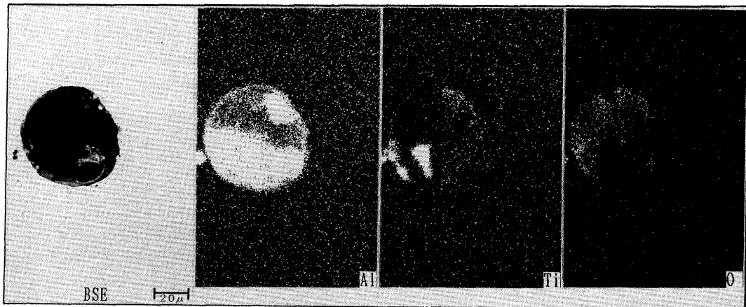
Fig. 7. EPMA image on the inside of a pinhole.
