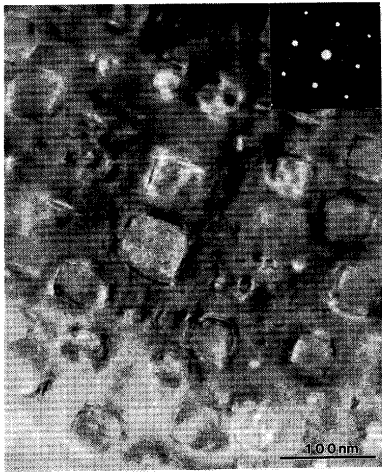
Fig. 3. TEM micrograph and selected area diffraction pattern of Alloy 706 stabilized at 780°C and aged.
