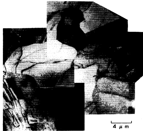
Fig. 3. TEM micrograph of the invar alloy annealed at 650°C x 53min.(Red. 78%)
