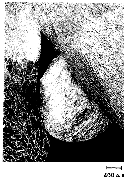
Fig. 7. The microstructures at the root of penetration beads with a sputter in the first layer.
