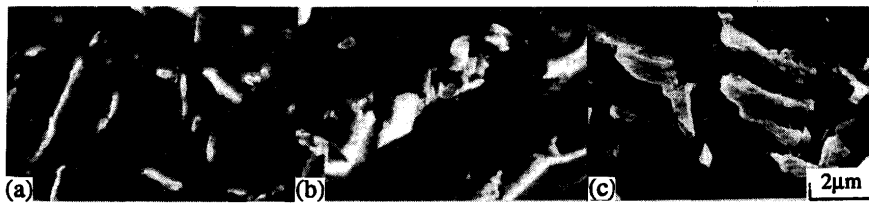
Fig. 4. SEM micrographs showing precipitation of the second phase particles in the steels tested. (a)0%Ni-T1 (b)0%Ni-T3 (c)4%Ni-T3
