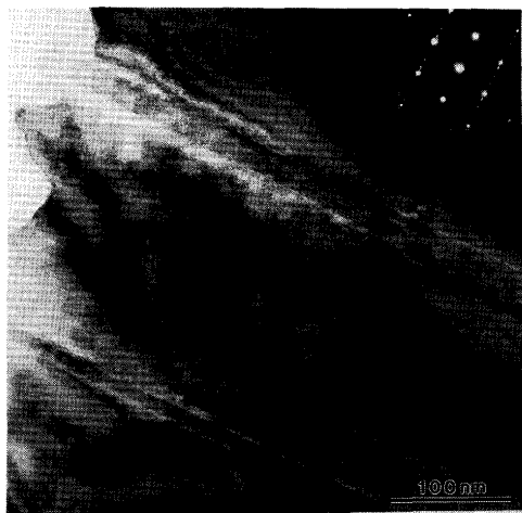
Fig. 4. A TEM micrograph and a selected area diffraction pattern near the grain boundary of experimental alloy No.4 aged at 830°C for 10h.
