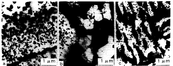
Fig. 7. TEM micrographs of 9Cr-7Mo-Ni steels crept at 923K.
