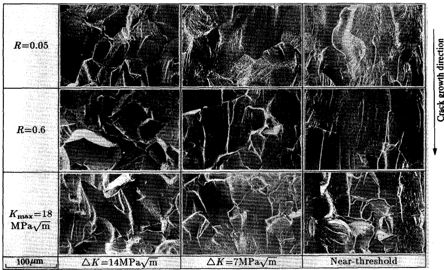
Fig. 9. SEM micrographs of fracture surfaces for STA850.
