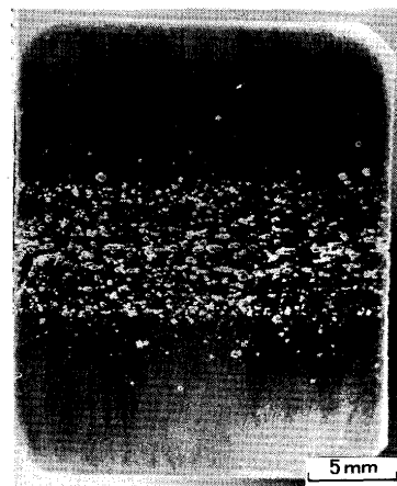
Fig. 9. Corrosion Morphology at Cross Section of Type304ULC SS in Coriou Test.
