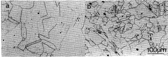
Fig. 10. Optical micrographs of the (a)SUS316 and (b)JPCA-2 cooled down to 77K after the solution treatment.
