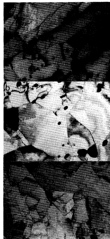
Fig. 5. TEM photographs of the aged JFMS. (a) 3.6 \times 10^3 , (b) 1.08 \times 10^4 , (c) 2.88 \times 10^4 ks.
